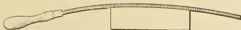
Fig. 49—How a thin file will bend when held in the manner shown in Fig. 48
